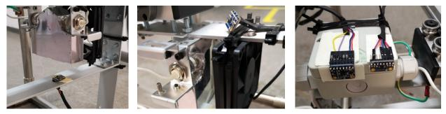
Figure 3: UV sensor under the UV lamp with reflector unit, temperature sensor next to the UV lamp, acceleration and temperature sensor in the upper part of the printing chamber (from left to right)
