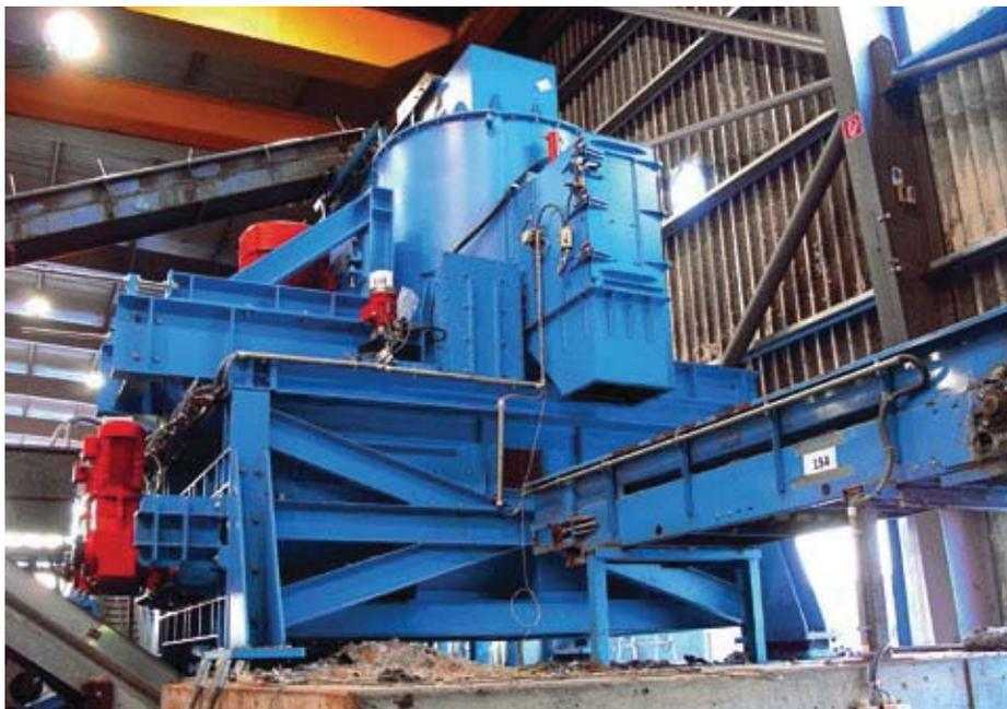
Abb. 1: Querstromzerspaner
