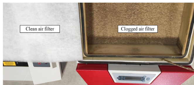
Fig. 2. Real image of a clogged filter of a laser cutting machine
