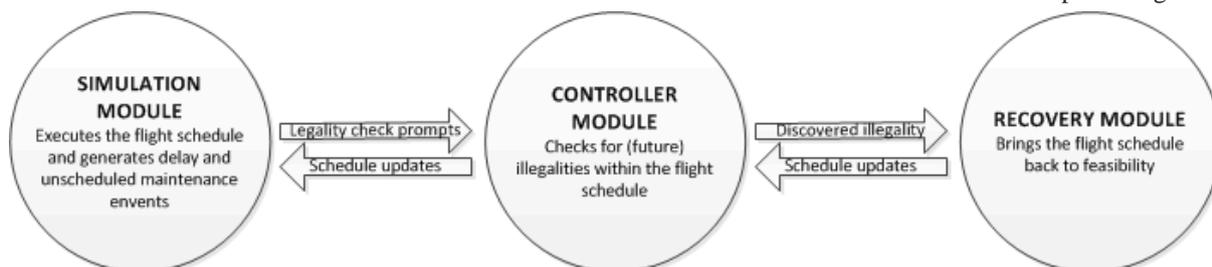
Figure 1. Modular simulation architecture of SIMAIR
