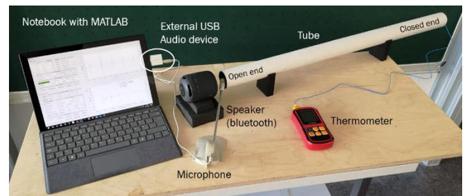
Figure 3: Equipment and experimental setup for use case 1
