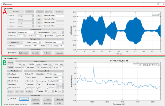
Figure 1: GUI of the MATLAB toolbox “Acoustics”. Section A: data acquisition settings and display. Section B: data analysis and presentation of results.
