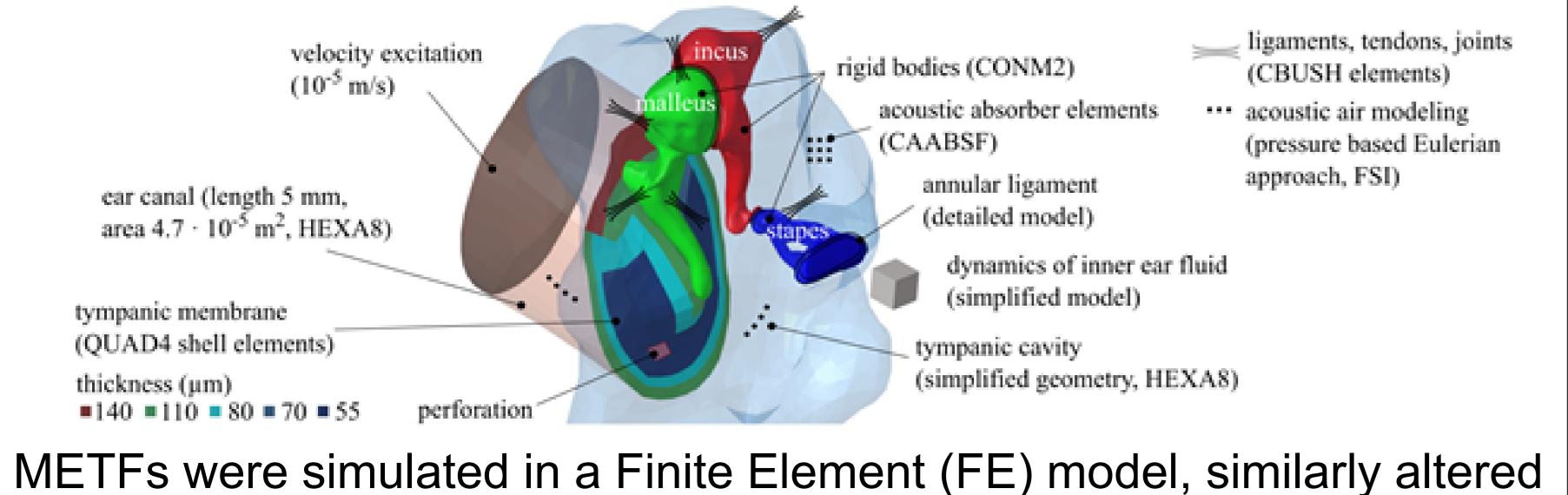
and compared to the measured METF data.<sup>3</sup>
