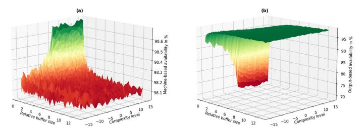
Figure 3. (a) Machine-based availability and (b) output-based availability over relative buffer size and complexity level.
