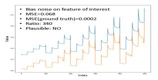
Fig. 12. Testing agent for predicting feature-1 based on 3 most related features. Bias noise on the FoI, MSE=0.068 (340x ground truth). (Blue: real data , Orange: predicted data)
