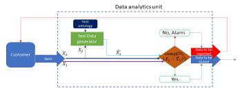
Fig. 5. Feature selection and decision making procedure in more details for the first solution.
