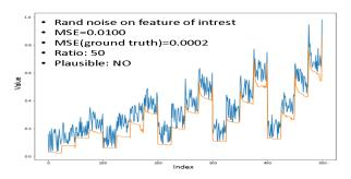
Fig. 13. Testing agent for predicting feature-1 based on 3 most related feature. Random noise on the FoI, MSE =0.01 (50 times higher than the ground truth). (Blue: real data, Orange: predicted data)
