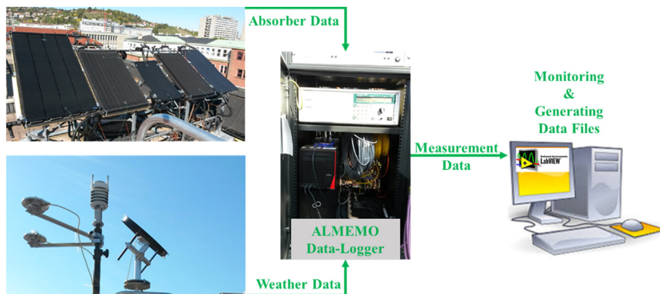
Fig. 1. The concept of data acquisition of the measurements at the test facility at HFT-Stuttgart.
