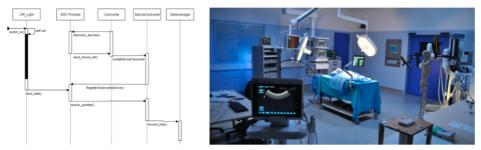
Figure 1. Sequence flow depicting how SDC data is transferred to the data management system (left) and mock operating room testbed for the system at Reutlingen University (right).
