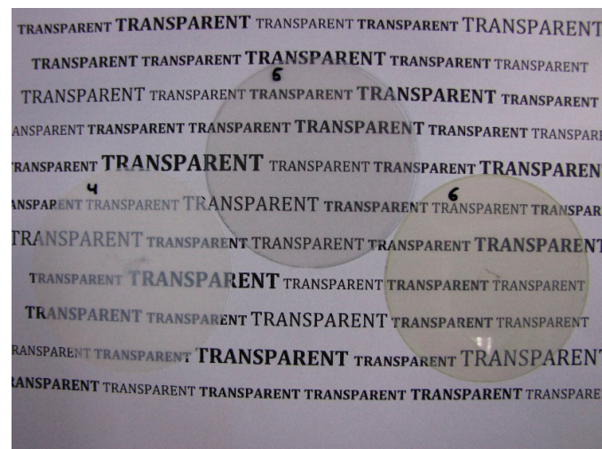
Figure 1. PET films spin-coated with three different TCO coatings. The left sample (4) is prepared with the AZO particles, the one in the middle (5) with ITO particles delivered as dispersion and the right one (6) with ITO powder dispersed by ultrasonic treatment.
