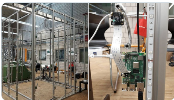
Figure 1: 3D Scanner installation.
