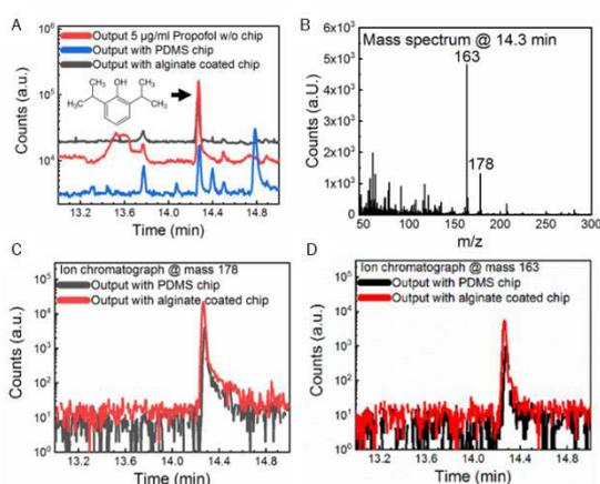
**Figure 3.** GC-MS of alginate coated microchip. A represents the chromatographs of flow system w/o chip (in red), pure PDMS chip (blue), and a PDMS chip coated with alginate monolayer (in black). B is a detailed mass spectrum of propofol peak at 14.3 min. C and D are extracted ion chromatograms, correspondingly  $m/z$  178 and  $m/z$  163, from uncoated (in black) and alginate coated (in red) samples.
