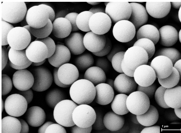
Fig. 7. FIB-SEM Image of Fu-Mel particles. The particles were sputter coated with 5–10 nm gold, and images were recorded using a charge reduction sample holder with an acceleration voltage of 3 kV.
