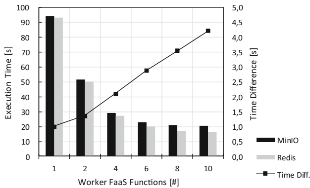
Fig. 8 Measured execution time of numerical integration application instance based on MinIO/Redis backend service
